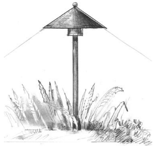
FIGURE 8: FULL-CUT OFF FIXTURE DIRECTS LIGHT DOWNWARD AND IS FULLY SHIELDED.
